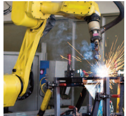
ARCAL 21 ensures high productivity and reduces spatters in robotic welding.
